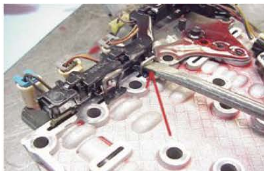
Figure 2: Removal of solenoid retaining clips
