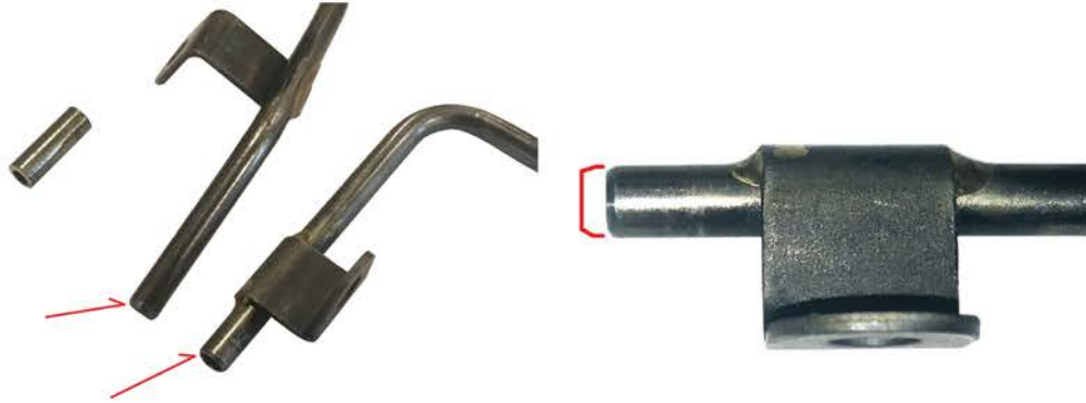
Figure 8: Tube after chamfering
